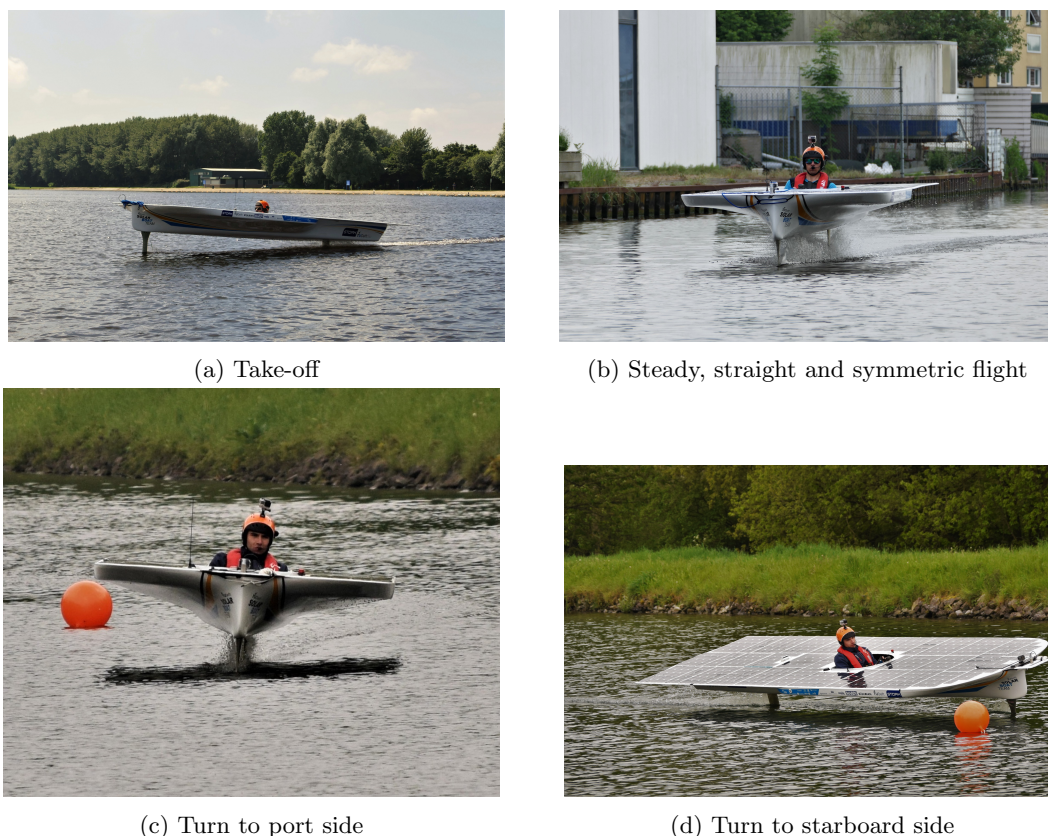
Figure 3: Four typical maneuvers of a single-track hydrofoil boat: the TU Delft Solar Boat 2016.
