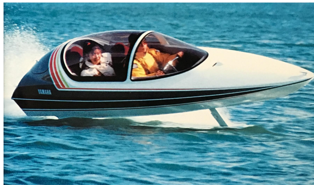
Figure 1: Kotaro Horiuchi has been designing and building single-track hydrofoil boats since the 1960's. Shown here is the OU32 single-track hydrofoil boat from 1988. From: [2].
