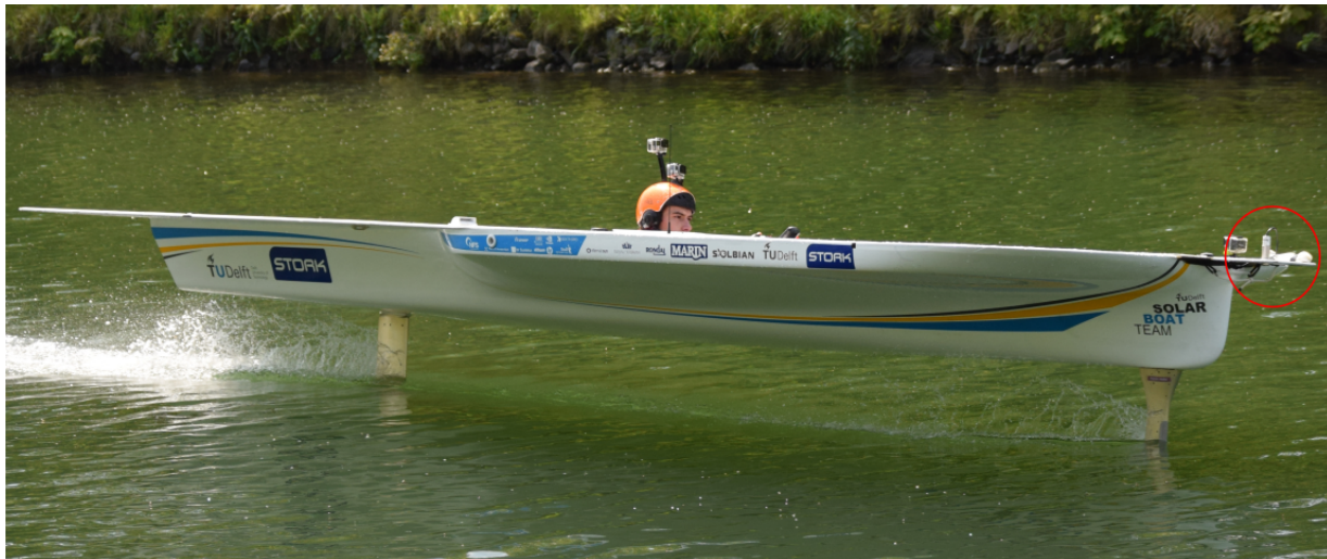
Figure 13: The Senix ToughSonic REMOTE 14 [12] constantly measures the height of the boat.
