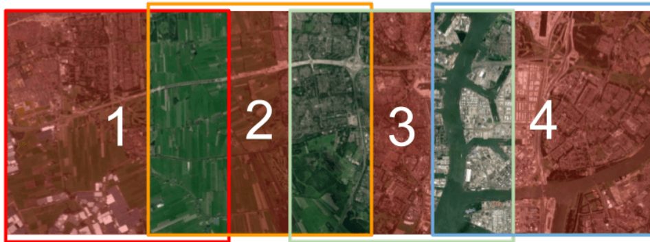
Figure 5.13: Four partly overlapping images, acquired by the sharpness sensor. Each area of overlap can be used for one sharpness optimisation step. Satellite image © DigitalGlobe.
